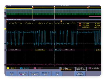
Figure 16. Triggering on specific Identifier and Data on a CAN bus and decoding all messages in the acquisition.
